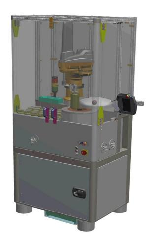
RoboCount™ LAB/20 can be operated in a manual mode. This mode is useful for measuring urgent samples, those with non-conforming geometry, calibration standards, or in the unlikely case of a software or hardware failure.
